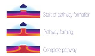
Over several minutes, the isothermal pathway forms under the sensor, bringing the core temperature to the surface.
