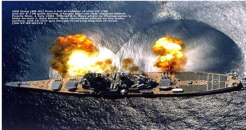
“Real life” reflecting surfaces make complex blast pattern – accumulates blast pressures
