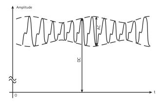
**Figure 3.** Graphic representation of raw infrared signal processed internally by the pulse oximeters, where AC represents the variable absorption of infrared light due to pulsating arterial inflow and DC represents the constant absorption of infrared light due to skin and other tissues.
