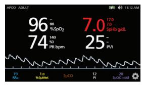
Figure 4. Screenshot of pulse oximeter display showing PVI numerical value and trend graph.
